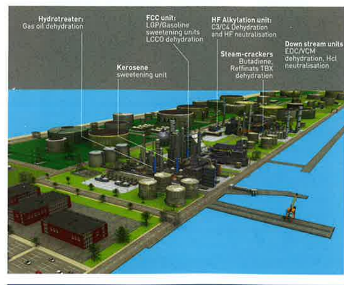
Figure 3. Solid drying in the petroleum industry.
