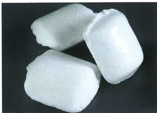
Figure 4. NaOH briquettes, weighing 29 g each.
